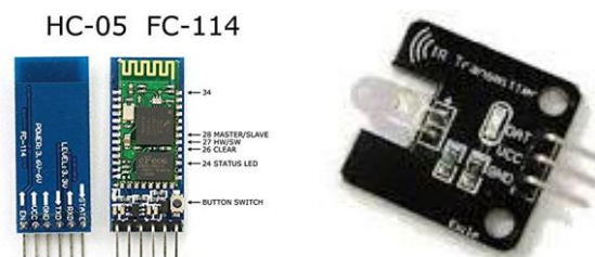
Figure 10. Bluetooth module (HC-05) + Infrared (IR-T940)
