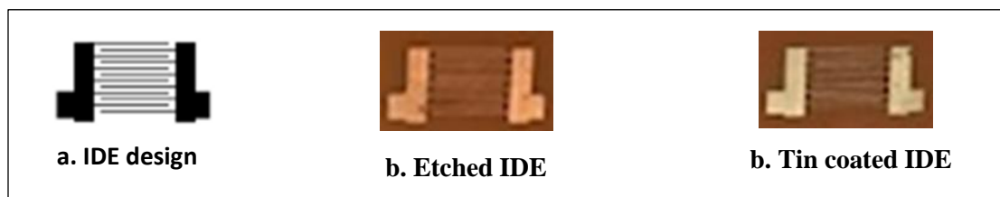
Figure 2 Stages in design and fabrication of IDEs
