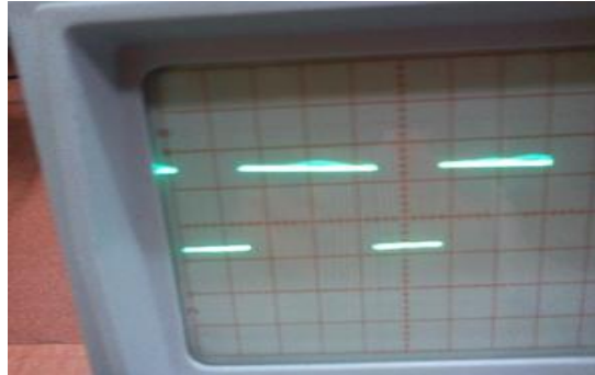
Fig14: Pulse generated from the driver unit (12V)
