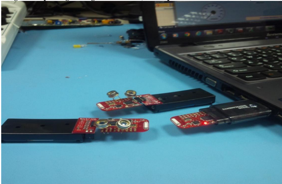
Fig 16 test bench setup using four sensors transmit the signal wirelessly
