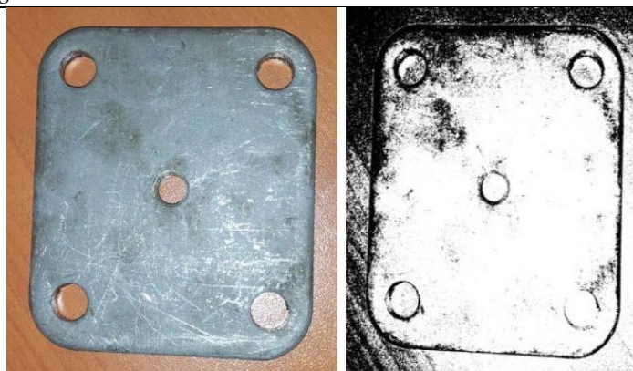
Figure 6: Actual product used for quality control with their binary image
