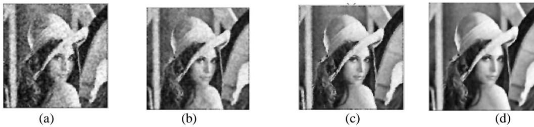
Fig. 3 Lenna image experiment (a) Restored image by lucy algorithm with wavelet analysis (b) Restored image by adjusted PSF (c) Restored image by combined approach (d) Final restored image based on gray transformation & filtering
