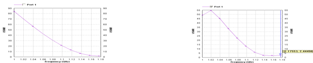
Figure 6 (a) Voltage Standing Wave Ratio of the proposed antenna before stacking (b) Return Loss of the proposed antenna after stacking
