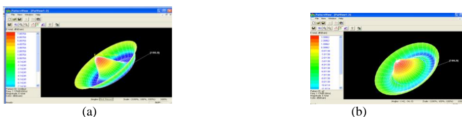
Figure 4. (a) Proposed antenna gain at 1.17645 GHz before stacking (b) Proposed antenna gain at 1.17645 GHz after stacking
