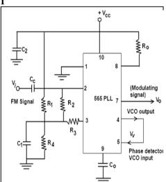
The input FM signal,  $V_i$ , is applied to pin number 2 through the coupling capacitor  $C_c$ . A part of this signal is also applied to pin number 3 through the potential divider network, consisting of  $R_2$ ,  $R_3$ , and  $R_4$ . The dc power supply is also provided to the input pins 2 and 3 through  $R_1$  from  $+V_{cc}$  supply. The capacitor  $C_2$  is used to filter out an AC ripple, if present in the DC supply.
