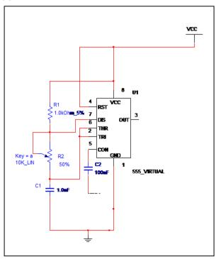
Pin 1 is grounded; pins 4 and 8 are shorted and then tied to supply +Vcc, output ( $V_{OUT}$ ) is taken form pin 3; pin 2 and 6 are shorted and the connected to ground through capacitor  $C_1$ , pin 7 is connected to supply +  $V_{CC}$  through a resistor  $R_1$ ; and between pin 6 and 7 a resistor  $R_2$  is connected. At pin 5 a bypass capacitor of 100 nF is connected.
