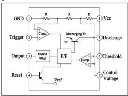
The block diagram of a **555 timer** is shown in the above. A 555 timer has two comparators, which are basically 2 op-amps, an R-S flip-flop, two transistors and a resistive network.
