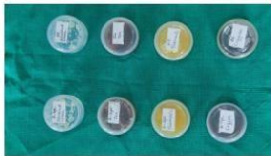
Fig. 5. Specimens immersed in their respective mediums (group I) – Ominichroma; Group II – GC Solar X
