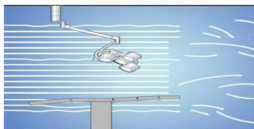
Fig1 Demonstration of vertical LAF ventilation
