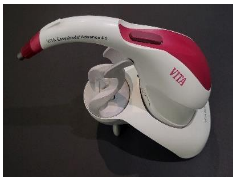
Vita Easyshade spectrophotometer Advance 4.00
