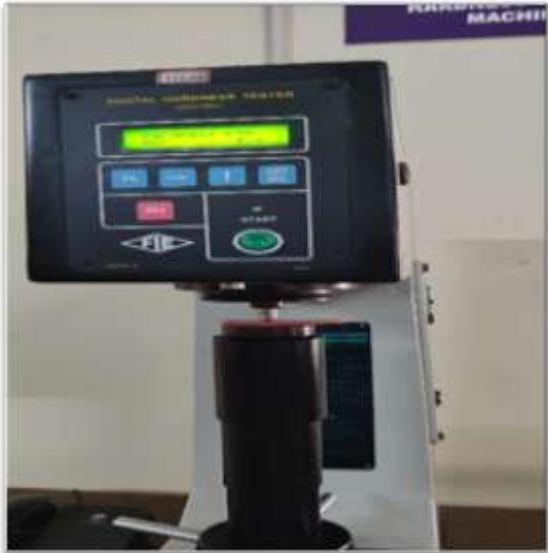
APPLICATION OF LOAD FOR TESTING HARDNESS USING ROCKWELL HARDNESS TESTER
