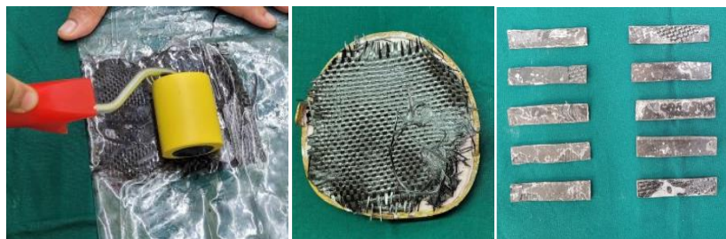
Figures: a: a roller was used to expel the air between the layers of carbon fiber; b: introduction of carbon fiber into the prefabricated mould; c: the processed carbon fiber in the predetermined dimensions
