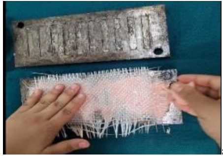
2) Adaptation of the pre-soaked e-glass fiber into the mould space along with heat-cure PMMA
