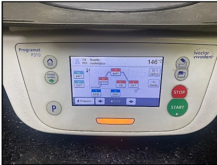
Figure (11): Firing cycle of Rosetta SM
