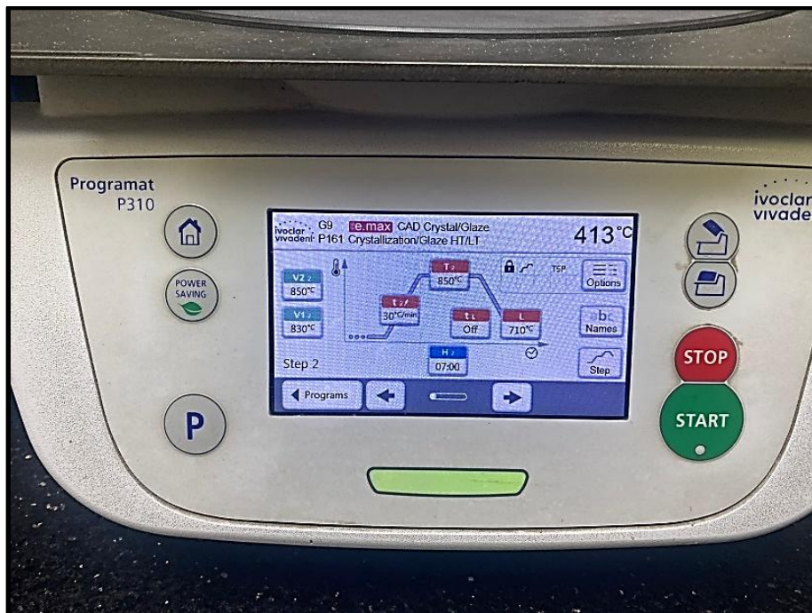
Figure (10): Firing cycle of E.max CAD
