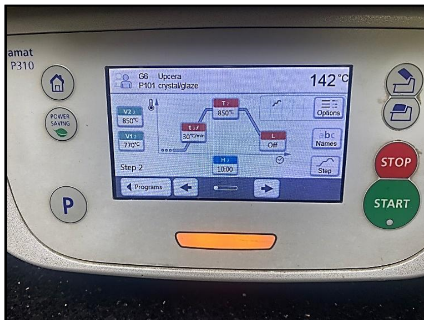
Figure (12): Firing cycle of Upcera CAD
