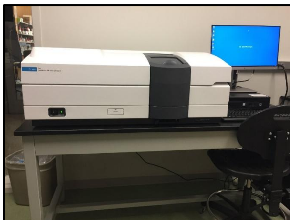
Figure (1): Backing the discs with white and black backgrounds using 'Agilent Cary 5000 spectrophotometer'
