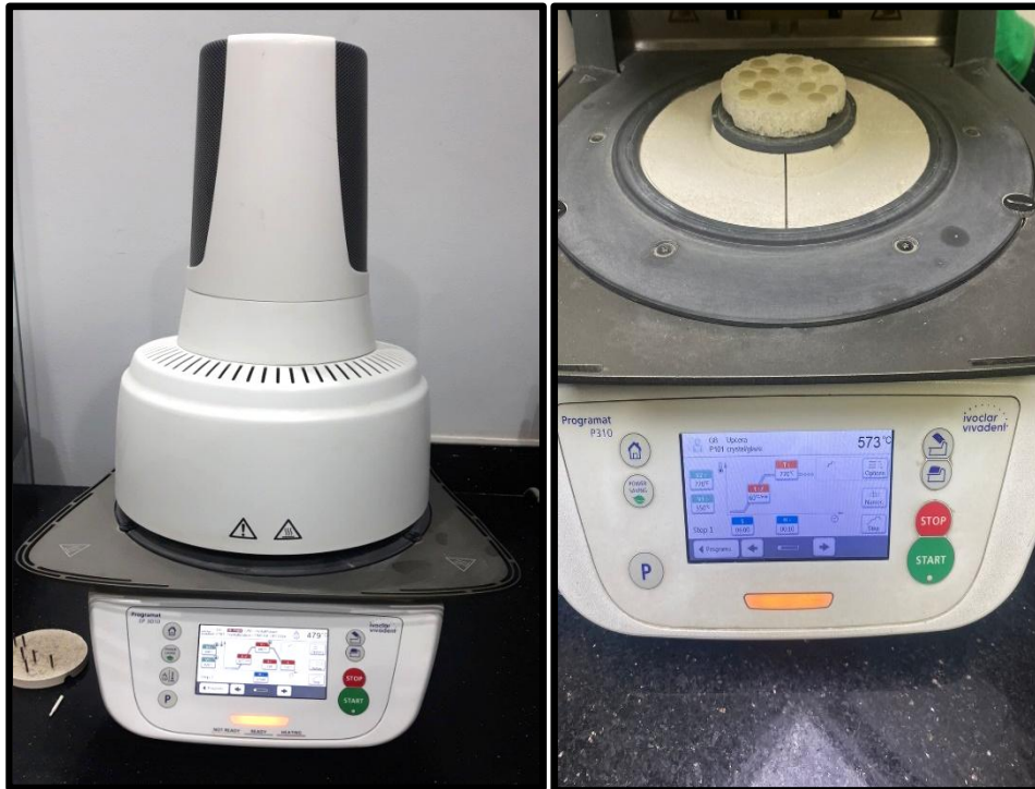
Figure (9): Glazing and crystallization of the specimens using Ivoclar Vivadent Programat P310 Furnace
