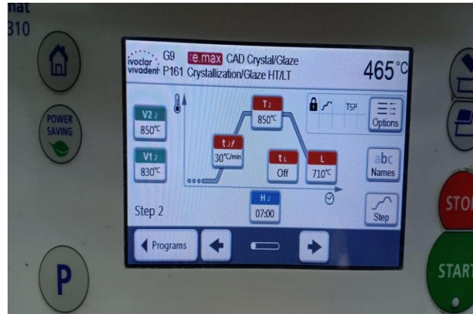
Figure (10): Crystallization cycle of e.max in programat p 310.
