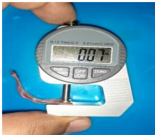
Figure 9: Measuring thickness of Dura lay using digital micrometer caliper
