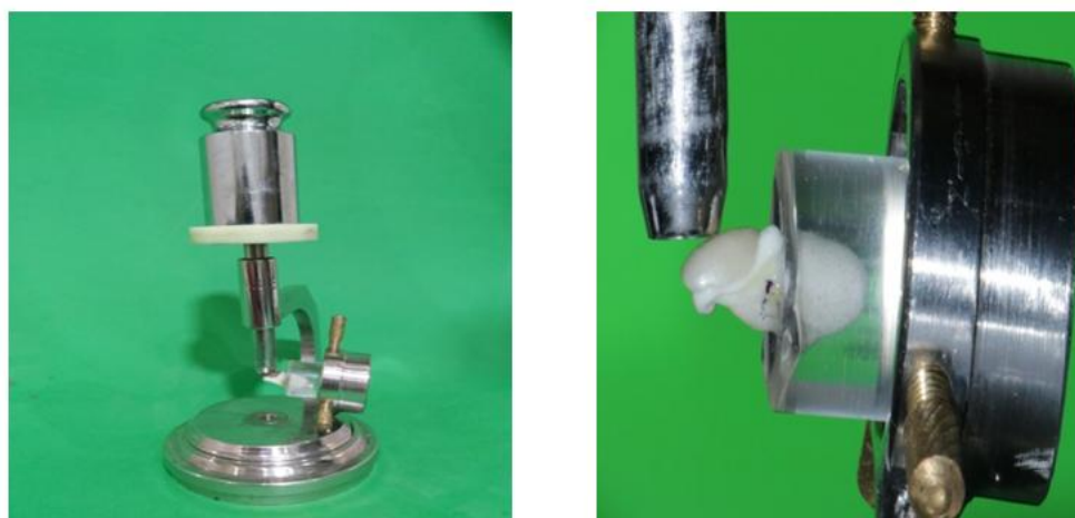
Figure 3: Showing specimen cementation in a specially designed loading device.
