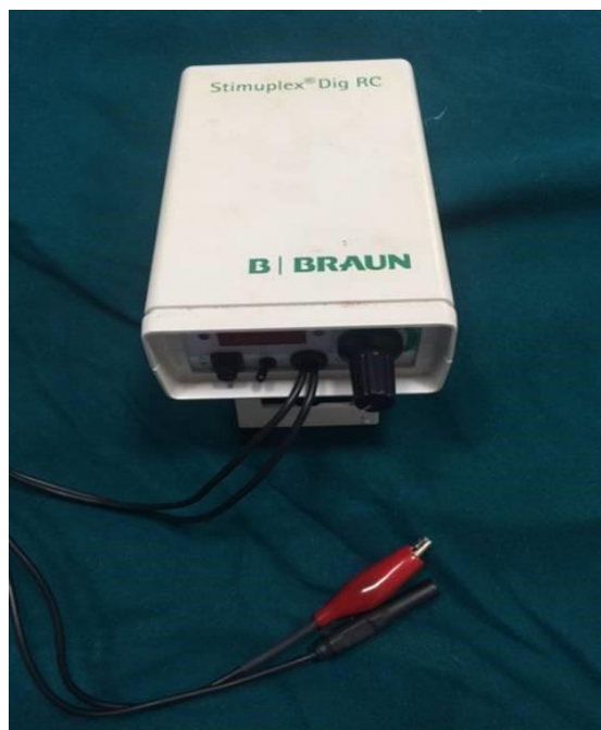
FIGURE NO 6: PERIPHERAL NERVE STIMULATOR.
