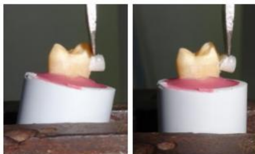
Fig 5: Prepared teeth samples under universal testing machine
