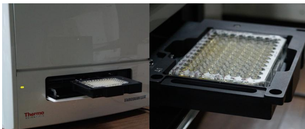
Figure 3: Absorbance value read at 600nm using Microplate Reader (Thermo Scientific Varioskan LUX)
