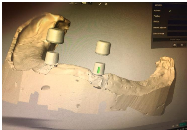
Fig 6: Final software design of secondary crowns.
