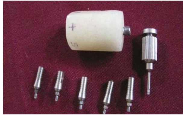
Figure.1. Five precision milled metallic standard abutments made of Grade 5 titanium (MD-MAC10, MIS Implants Technologies Ltd, Israel).
