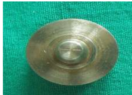
Fig3. Top View Of Master Die Showing Horizontal groove.
