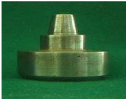
Fig2 Steel Master Die: Showing Vertical Groove
