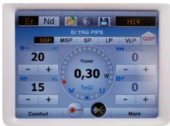
Fig.3:- Touch screen panel showing the PIPS setting, at 20 mJ, 15 Hz, no air / no water, 50 microsecond pulse duration.
