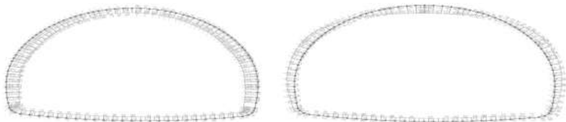
Figure 11. The state of a) axial force and b) bending moment in tunnel lining under static loading (FZ section)
