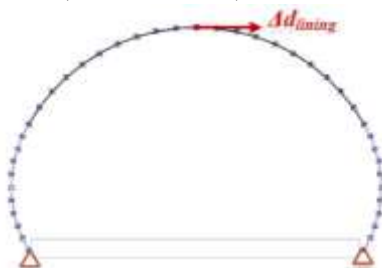
Figure 5. Loading condition for earthquake loading
