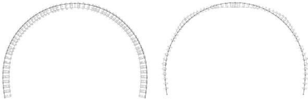
Figure 9. The state of a) axial force and b) bending moment in tunnel lining under static loading (E at section)
