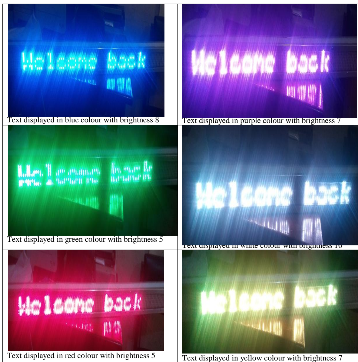
Fig. 3: Different Display of Text, Colour and Brightness
