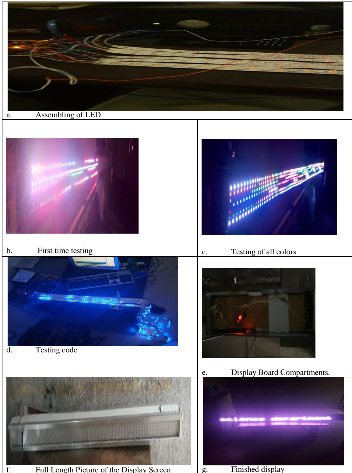
Fig.2: Assembly and Testing of LED Strip Light
