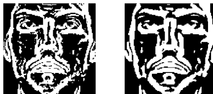
Figure 4–Sobel gradient detection comparison with 3x3 pixel kernels [left] and 7x7 pixel kernels [right].
