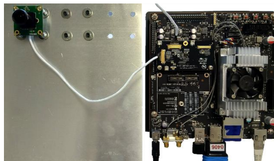
Figure 11 - Nvidia Jetson TX1 dev kit and Leopard Imaging camera used for our embedded smart video surveillance system.
