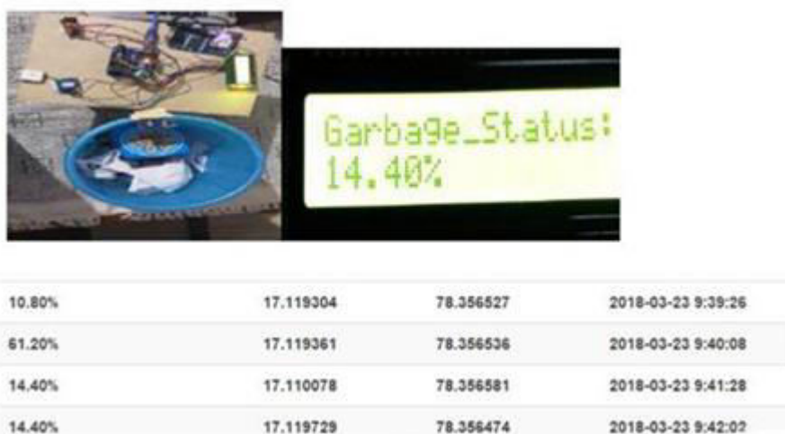
Figure 16. LCD displaying the status with percentage left empty in Garbage Bin
