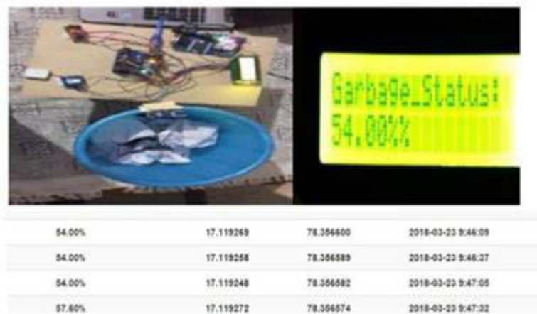
Figure 15 LCD displaying the percentage of space left in Garbage Bin
