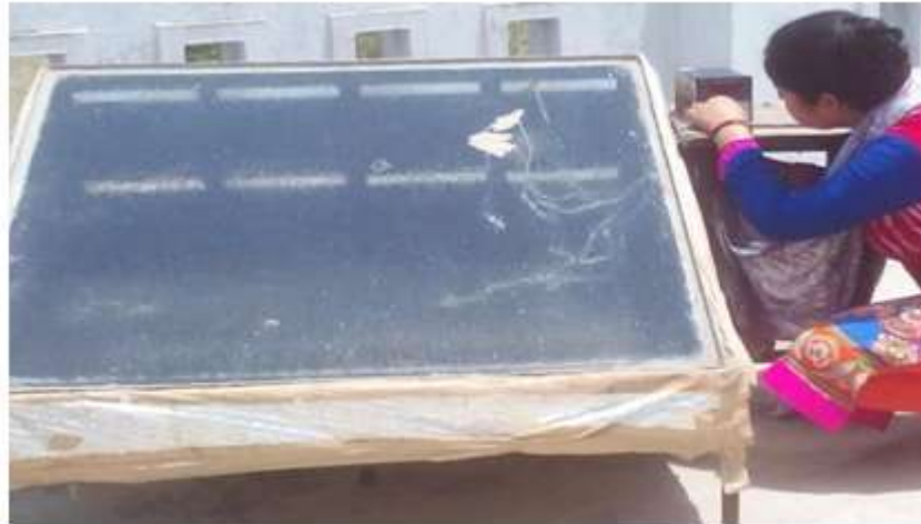
Figure 1 Experimental setup of still with separate condenser.
