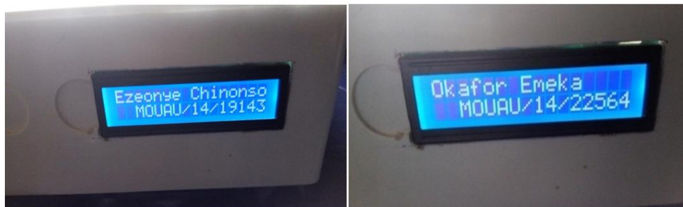
Plate 2: LCD Display when card is swiped
