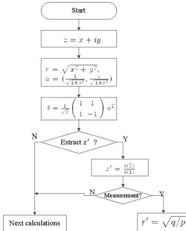
**Figure 3.** Program flow chat of quantum computing simulation of complex operator  $z' = \frac{1-z}{1+z}$ . In the figure p is the measurement possibility of state  $|0\rangle$ , and q, state  $|1\rangle$ .
