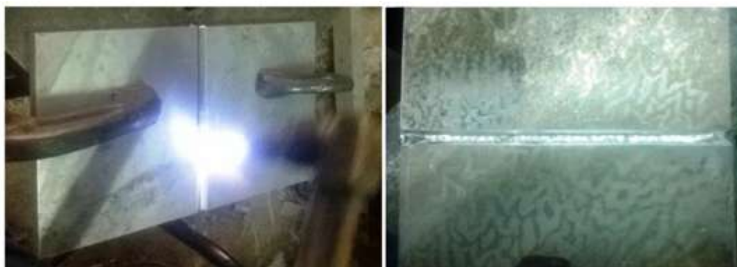
Figure 1 Aluminum plates are preheating and welded.
