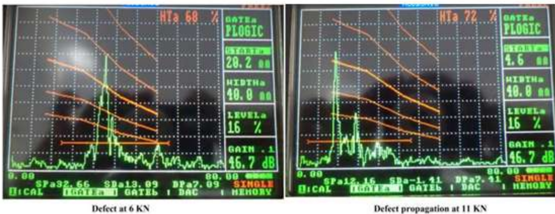
Figure 8 Defect propagation in defect weld sample due to increase in load.
