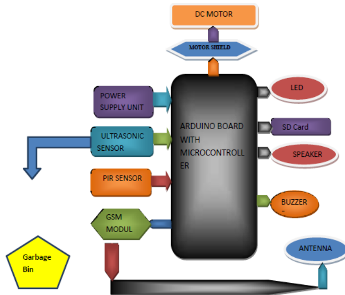
Figure 1: block diagram of the proposed system at transmitter side
