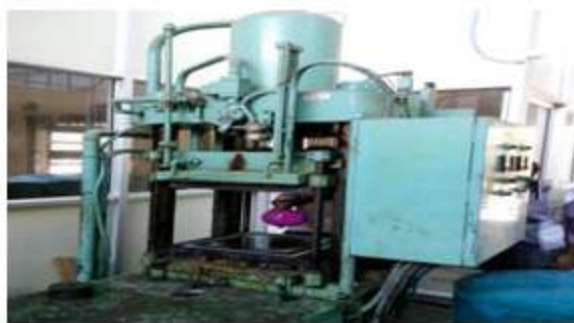
Figure 3 Compression moulding machine used for biocomposite.
