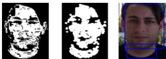
Figure 9: Skin color results (left: binary image, middle: morphological conversion, right: drawn outline)
