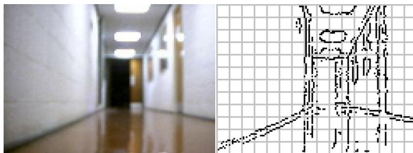
Figure 6: Pre-processed image broken down into 8x8 sized sub-images
