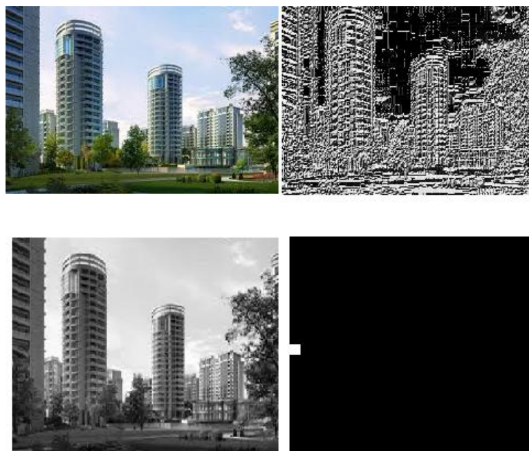
Fig. 3: (a) Original image, (b) CS-LBP extracted feature representation, (c) forged image, (d) shows the generation of mask of forged area in the image.
