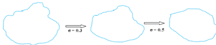
Figure 3: Smoothing process for a curvature at different smoothing factors.
