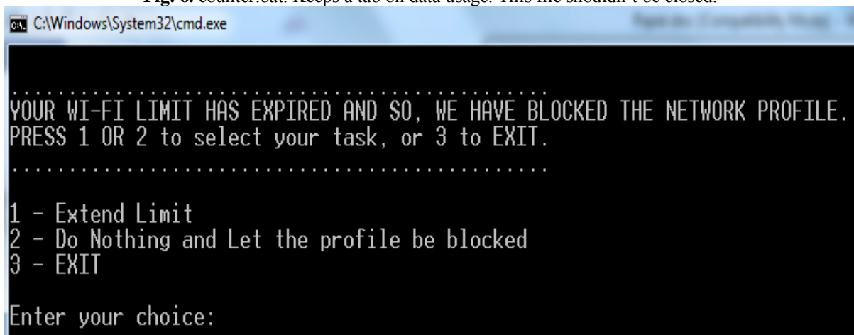
Fig. 7(a). run_2.bat. As soon as the limit gets exceeded, counter.bat calls on run_2.bat to allow user to modify the limit. Option 2 and 3 are used to exit the program.
