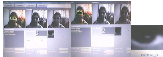
Comparison between haarcascade_frontalface_alt2.xml (eigenface) and haarcascade_eye.xml (eigeneye) files Eigenface eigeneye
