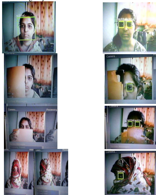
Comparison between haarcascade_frontalface_alt2.xml (eigenface) and haarcascade_eye.xml (eigeneye) files Eigenface eigeneye
