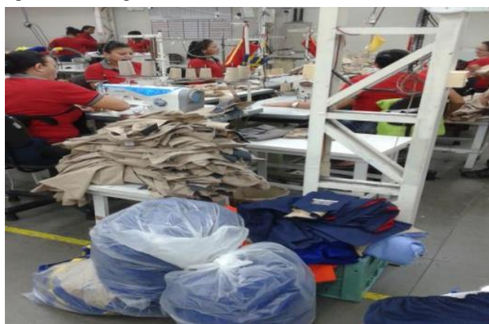
Figure 4: Multiple batches of production halted and insertion of different items in the same cell.
