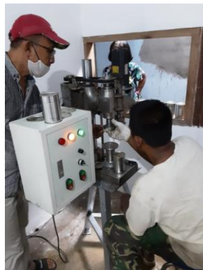
Figure 4: Automatic seamer machine, capacity 120 cans per hour
