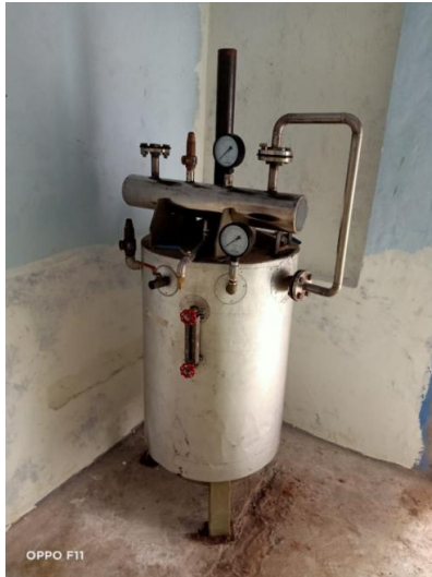
Figure 2: Boyler 4 bar heat generating engine.
