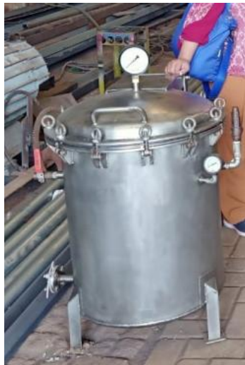
Figure 3: Autoclave machine with a capacity of 100 cans
