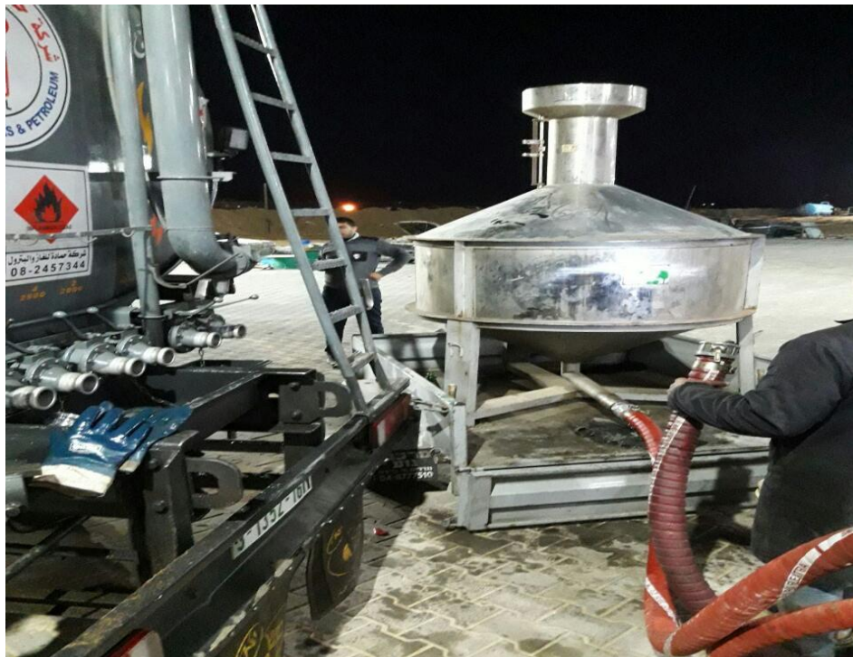
Figure (5) Calibration chamber and petrol vehicle during calibration. Source: researchers.
