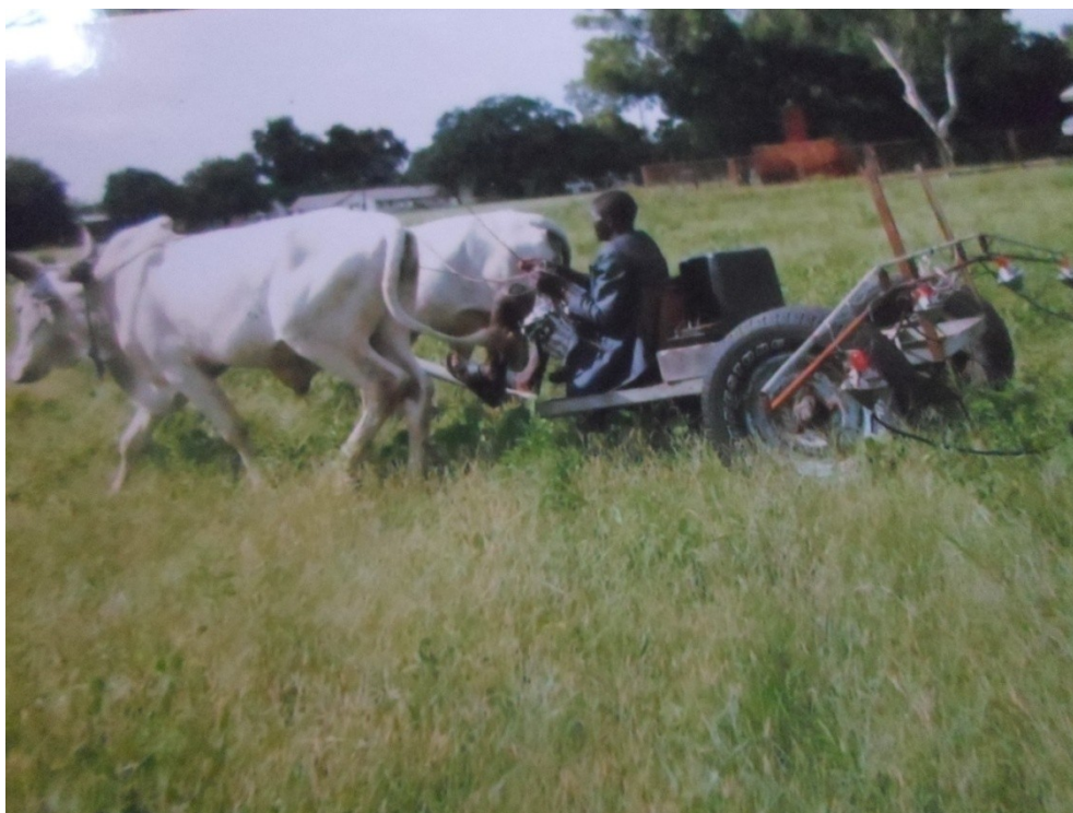
Plate: 2 Animal Drawn Ground Metered Shrouded Disc Sprayer during test-run
