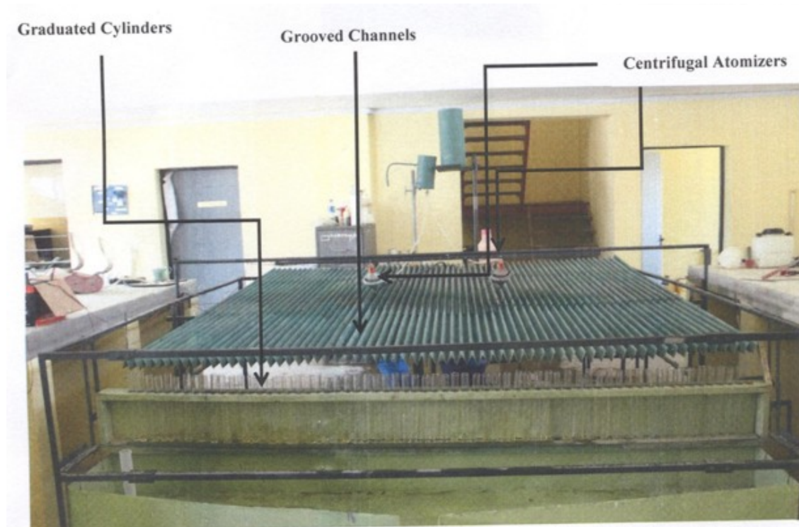
Plate 1: Patternator designed and fabricated by Enaburekhan (1981) at IAR Crop Protection Laboratory, ABU, Zaria
