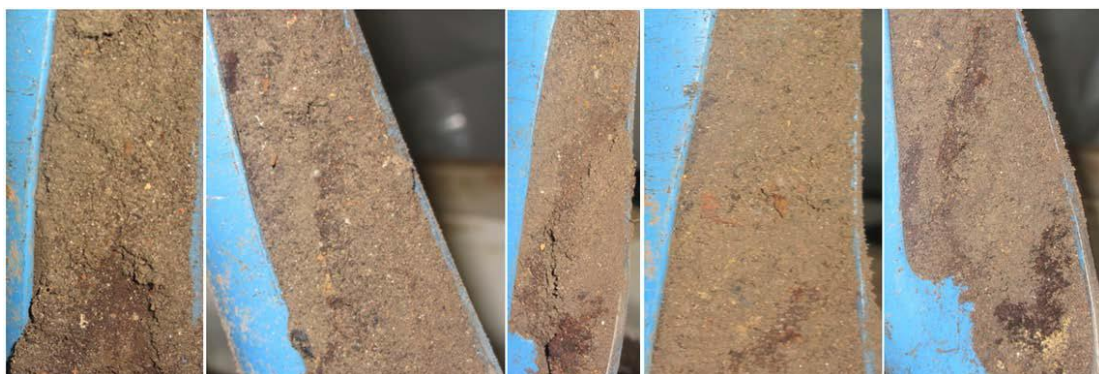
Figure 7. Changes in color and composition of soil profile samples taken randomly in a termite test tank after exposure to termite foraging.
