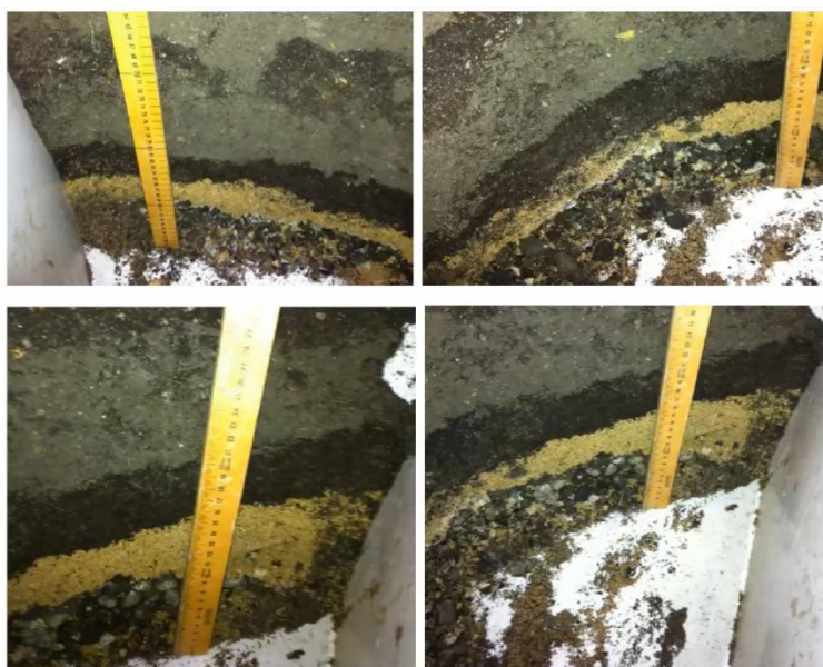
Figure 8. Views of a random soil profile cross section cut through a soil profile in a test tank.
