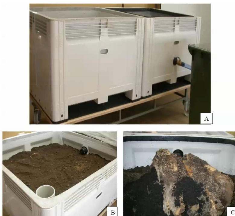
Figure 1. External view of termite ( C. frenchi ) test tank (A), top view of foraging tank after the establishment of the soil layers (B) and termite nest on the nesting tank (C).
