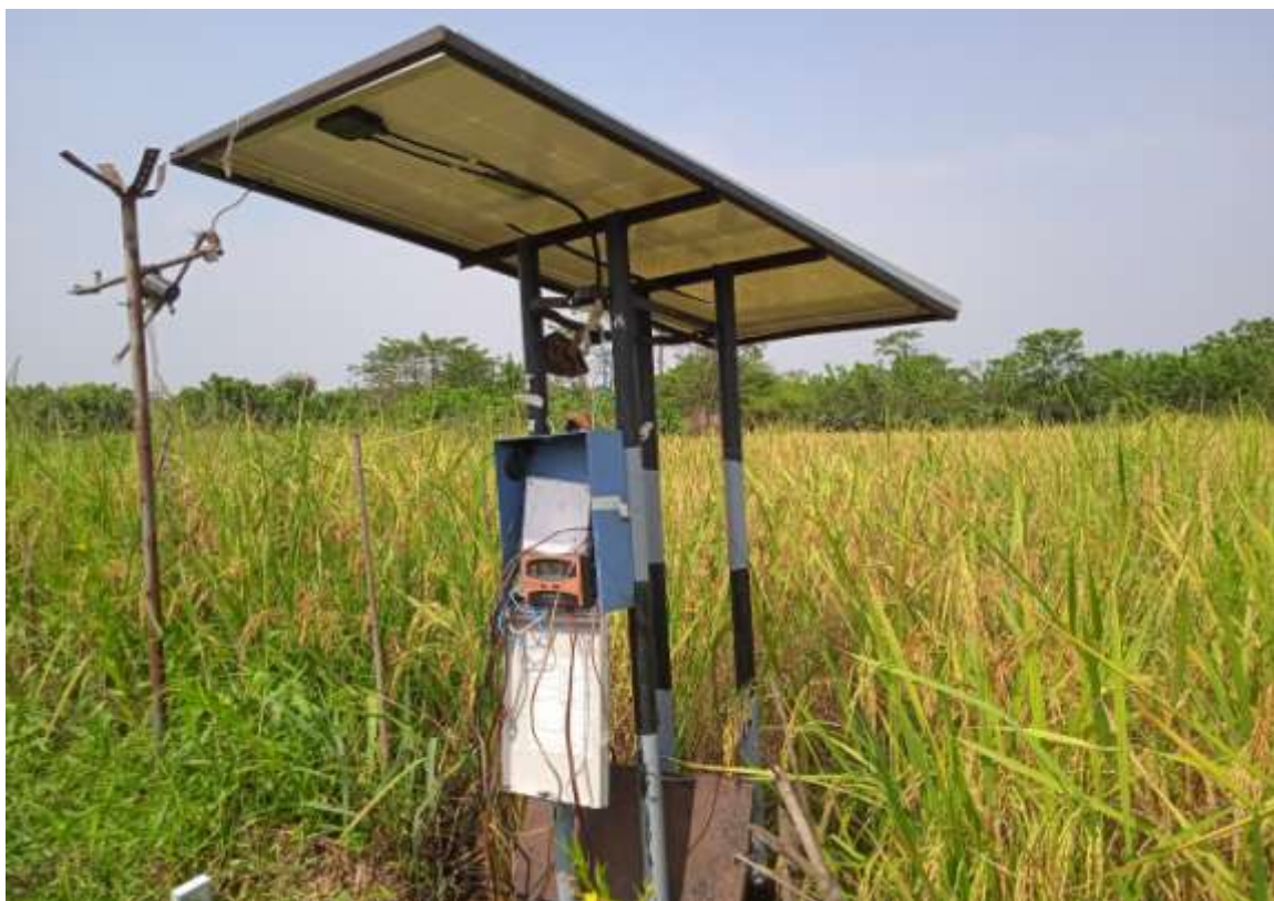
Figure 3: Deployed Solar Powered Pest Detection and Control System
