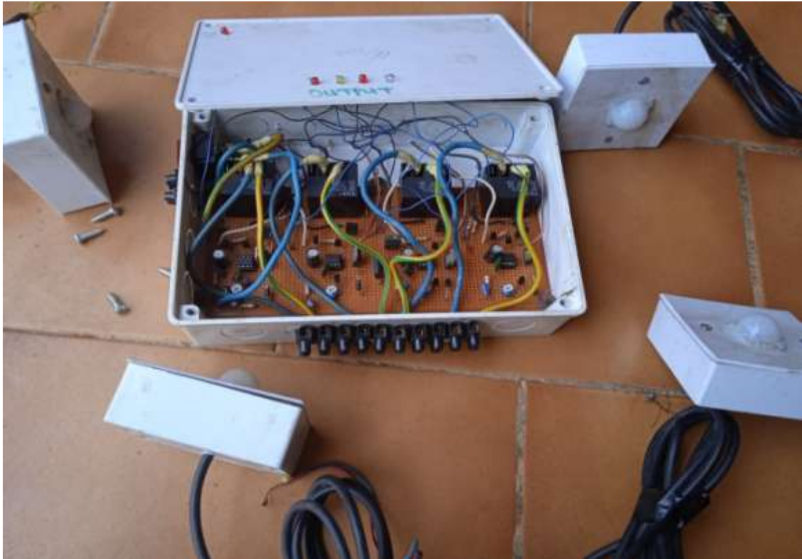
Figure 2: Developed control unit of Solar Powered Pest Detection and Control System [10]
