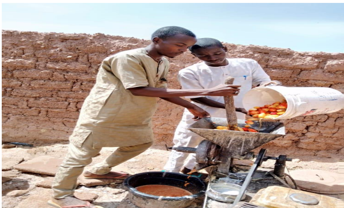
Fig. 2. Crushing and grinding fresh tomatoes and sweet pepper into raw paste
