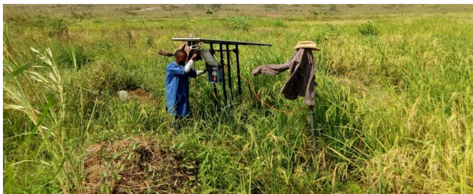
Figure 3: Field deployment of solar powered pest control system
