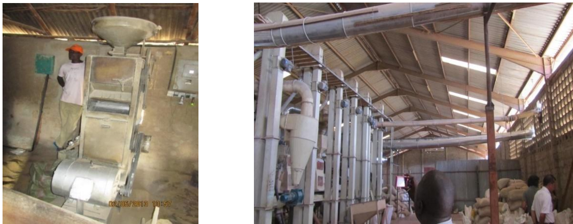
Figure 3: Single pass mill in Anyiko- Siaya (left) and Multi stage mill at MRGM- Mwea (right)
