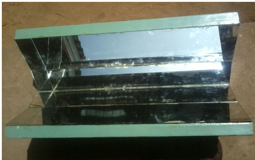
Figure 2.6: Mounted v-trough reflectors
