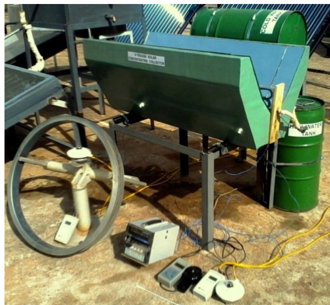
Figure 3.2: Diagram of the Test Loop/Experimental Setup
