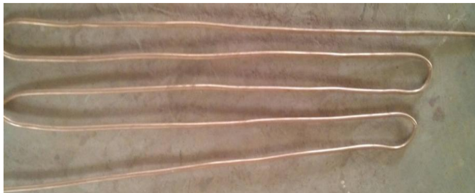
Figure 2.7: Copper Pipe Bent into Serpentine Shaped Passage
