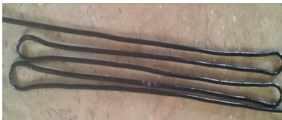
Figure 2.8: The Exposure Area of the Serpentine Copper Tube Painted Black
